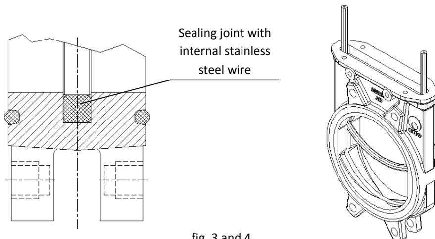
This rubber joint is inserted inside the body in such a way that it starts on one side, level with the packing, and continues around the body to reach the other end of the packing area.
