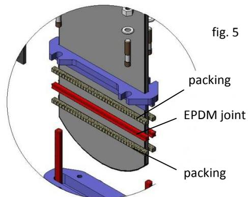
**GREASED COTTON (Recommended for hydraulic services):** This packing is composed of braided cotton fibres soaked in grease both inside and out. It is for general use in hydraulic applications in both pumps and valves.
